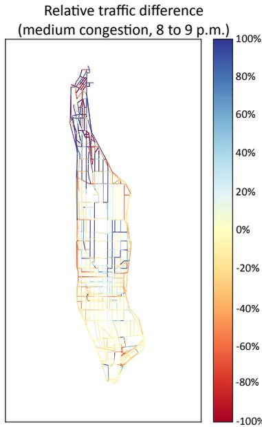
**Fig. 3** Performance of the “real-time congestion-aware rebalancing algorithm” as compared to the baseline algorithm in (Zhang and Pavone, 2016). The color of each road corresponds to the percent *difference* in the number of vehicles traversing it between the congestion-aware and baseline rebalancing algorithms—blue indicating a reduction in congestion using the congestion-aware algorithm.
