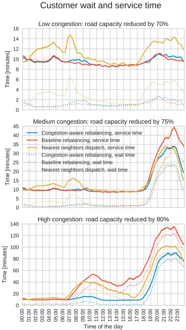
**Fig. 4** Comparison of customer wait and service times from different rebalancing and dispatching algorithms for low, medium, and high levels of congestion. The congestion-aware algorithm recovers the asymptotic behavior of the baseline rebalancing algorithm for low levels of congestion, and it outperforms both the baseline rebalancing algorithm and the nearest-neighbor dispatch algorithm for high levels of congestion.
