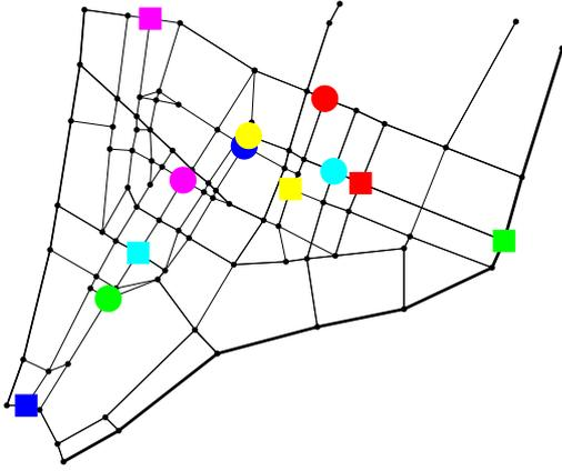
**Fig. 1** A road network modeling Lower Manhattan and the Financial District. Nodes (denoted by small black dots) model intersections; select nodes, denoted by colored circular and square markers, model passenger trips' origins and destinations. Different trip requests are denoted by different colors. Roads are modeled as edges; line thickness is proportional to road capacity.
