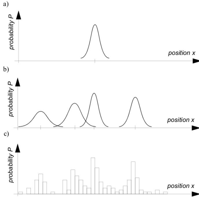
Figure 2: A graphical representation of different types of probabilistic representations: (a) a continuous single-hypothesis belief (e.g. from a single Gaussian distribution), (b) a continuous multiple-hypothesis belief (e.g. a mixture of Gaussians), (c) discrete representation with a finite number of possible values [SNS11].
