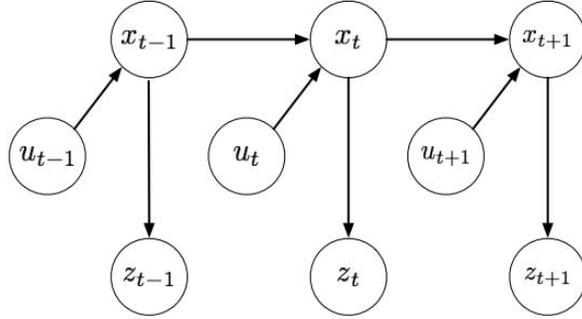
Figure 3: Graphical representation of the Bayes network model (hidden Markov model). Note that the sequencing assumes that the control is applied, and then a measurement is taken.
