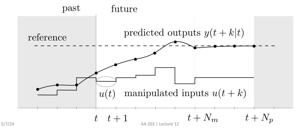
• Model predictive control (or, more broadly, receding horizon control) entails solving finite-time optimal control problems in a receding horizon fashion
