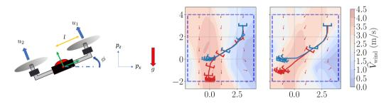
We compare ARMPC (blue line) to non-adaptive tube MPC (red line), with wind straight down from above (left) and wind at an incidence angle of 22.5 degrees (right). Tube MPC causes the drone to drift significantly, while ARMPC quickly learns to compensate for the wind drag (Sinha et al., 2023).
